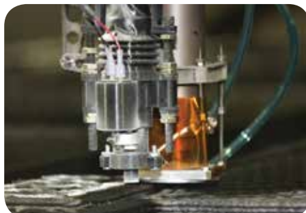
An extrusion screw for Big Area Additive Manufacturing (BAAM) can deposit material 200 times faster than existing systems.
