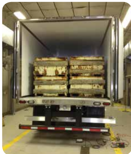
Structural Composites' all-composite truck body is designed for the refrigerated truck market.
